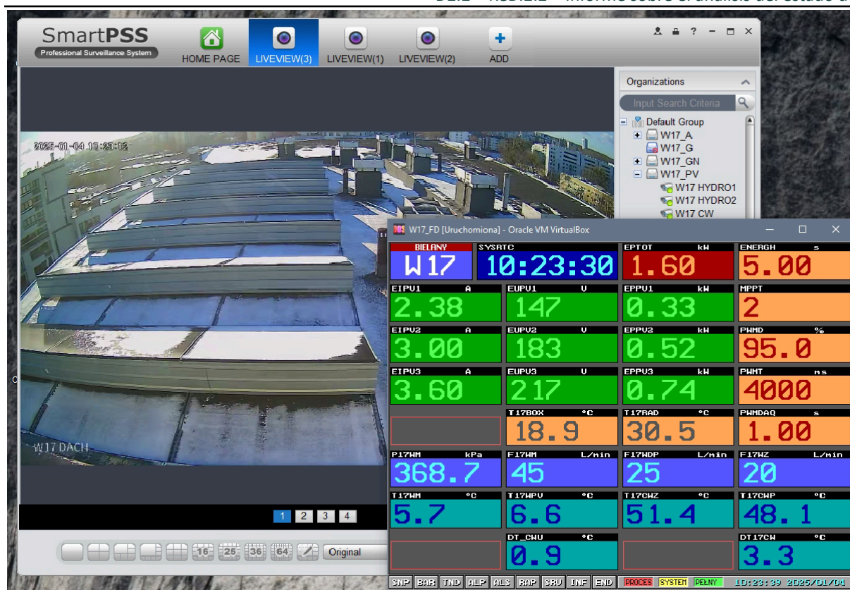
Figure 2. SCADA system monitoring photovoltaics on the roof
